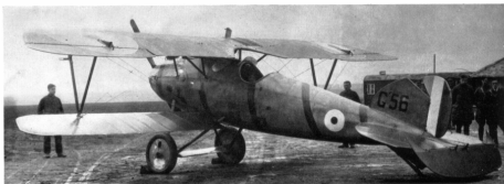
Captured Albatros D V, D2129/17, with spiral ribbon marking. Note British A.S.I. pilot head on port interplane struts.
