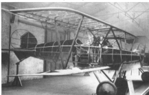
Captured Albatros D Va stripped of engine and fabric covering for display in London during 1918.
